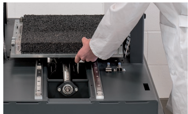
500 x 400 mm slab and lead rolled ball screw system
