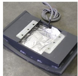
Heating system incorporated in mould base support
