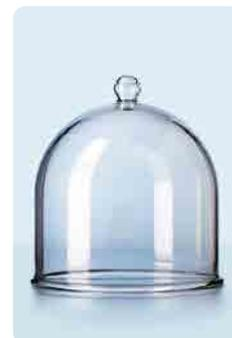
Wall thickness and geometry designed to suit vacuum applications. Neck aperture, standard ground joint NS 34/35.
