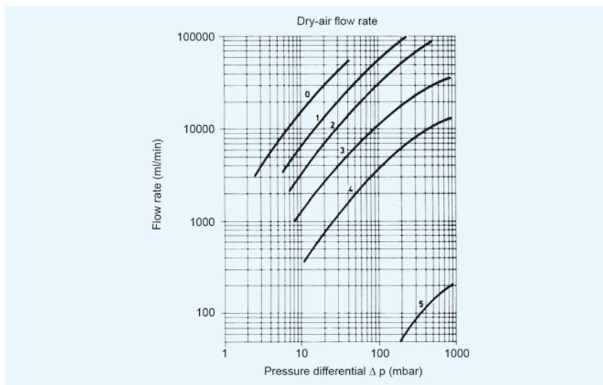
Air flow rate through filter discs of various porosities as a function of pressure differential. For filter discs with  $\varnothing$  30 mm
