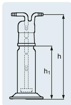
Typical applications: cleaning ("washing") of gases with solvents.
