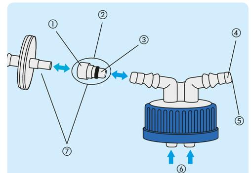
Screw cap GL 45 with 2 hose connections
