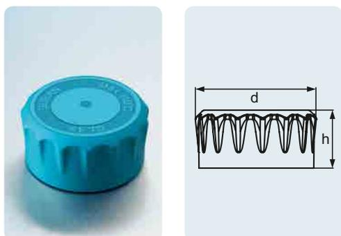
The DURAN® YOUTILITY Screw Cap GL 45 is manufactured from a food-grade polypropylene (PP). Ergonomically shaped screw cap with optimised grooves and ridges for a more efficient and easier tightening or removal. The faster opening and closing thread of the YOUTILITY screw cap is fully compatible with DIN GL 45 bottle threads. The optimised cap sealing system ensures a liquid tight seal. A pre-defined labelling area on the cap is compatible with the dedicated DURAN® self-adhesive YOUTILITY labels.
