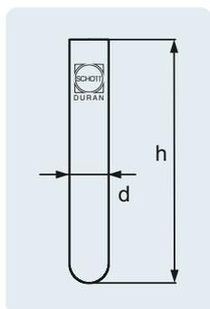
Centrifuge tubes are very resistant to mechanical loading. The higher density fraction collects in the bottom. Consequently solids can be collected and separated.
