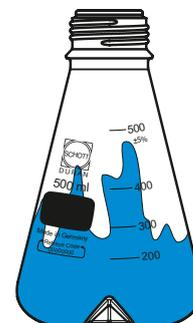
The movement causes a liquid sickle to form when using DURAN® Erlenmeyer flasks on a vibrator. The DURAN® baffled flask with four baffles on the bottom disrupts the laminar flow and produces a turbulent flow. The surface area of the liquid and the gas-exchange area are increased, thereby increasing the oxygen intake.
