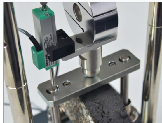
Detail of the integrated load cell and displacement transducer
