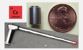
Cs-137 source is located at the tip of the source rod, pushed down by a handle. It can be used at various depth for Backscatter or Direct Transmission density measurement methods.
