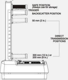
For all gauge models it is highly recommended to set the count time to 1 minute for good precision, or 4 minutes for best precision of measurement results. It is not recommended to use the shorter 15 seconds count time due to much lower accuracy.
