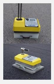
The 4640-B gauge is placed on the air gap spacer on the magnesium standard plate.
