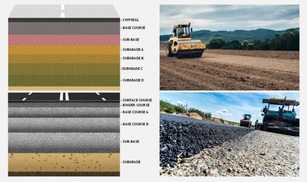
To determine appropriate level of compaction for different layers, various lab tests are employed. Most common one for soil is the Proctor test, also known as the Standard and Heavy compaction tests under NZS 4402.4.1.1 and 4402.4.1.2. These test methods cover the determination of dry density and water content relationship with the goal of plotting the Maximum Dry Density (MDD) and Optimum Water Content (OWC).
