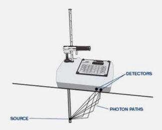
In the Backscatter mode, the radioactive source is lowered to position where it nearly touches but does not penetrate the surface of the test material.
