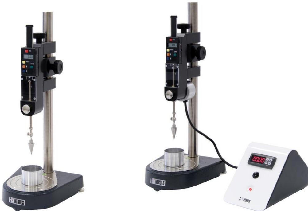
22-T0029/D: Digital liquid limit penetrometer with micrometric vertical adjustment
