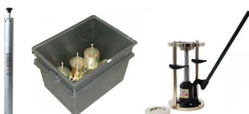
**33-T0075/B:** BS Standard compaction rammer, 2.5 kg
