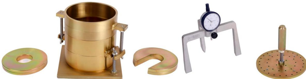
**G-T0090/PNZ:** CBR Mould Complete with perforated baseplate
