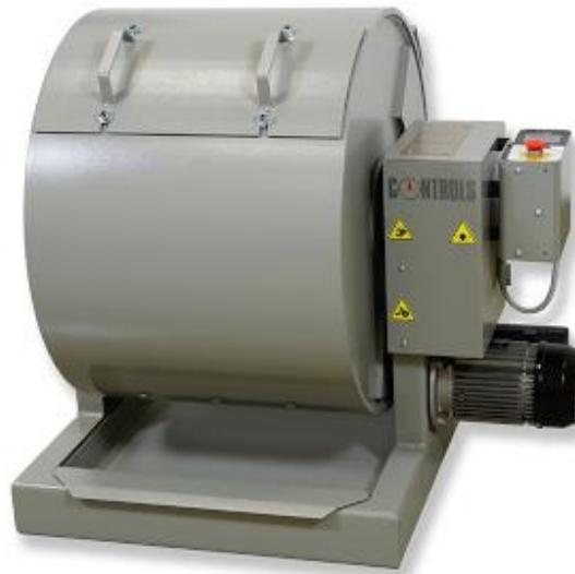
**48-D0500/G:** Los Angeles abrasion machine with graphic display and membrane keyboard
