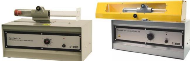
**47-T0056/B:** Motorized sand equivalent shaker
