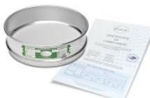
**200SIW1.70:** 200mm dia. x 1.70mm Stainless Steel Woven Wire
