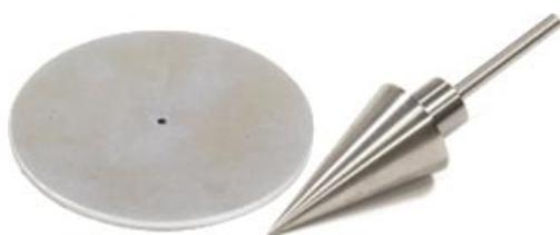
22-T0029/1: Penetration cone 30° tip and 80g of weight, to EN 17892-12, CEN ISO/TS 17892-6 and -12 and BS 1377-2
