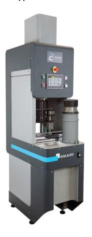
**78-PV20G02**: Galileo, fully electromechanical gyratory compactor Gyratory angle range: 0 - 3 deg,  $\pm$  0.01 accuracy Manual angle set-up and adjustment 230 V, 50/60 Hz, 1 ph
