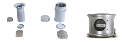
**78-PV0250/5**: Hardened cylinder mould 100 mm diameter, complete with top and bottom plates **78-PV0250/2**: Hardened cylinder mould 150 mm diameter, complete with top and bottom plates **78-PV0250/6**: Distance piece, 100 mm diameter, 38 mm high, for preparing short samples **78-PV0250/3**: Distance piece, 150 mm diameter, 50 mm high, for preparing short samples
