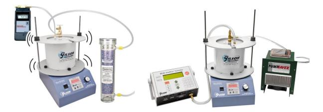
**SGA-5R**: Rice Shaker for Specific Gravity & Asphalt Rice Test 115V / 50-60Hz / 2Amps
