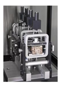
**79-PV72Q02/I2**: AsphaltQube, 15 kN modular electro-mechanically operated asphalt mix tester with inbuilt IMACS2 controller 208-230V/50-60Hz/1ph
