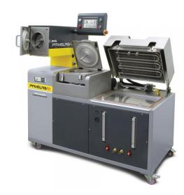
**75-PV50A15**: PAVELAB50 Automatic Closed-System Asphalt Analyzer for separation and extraction of bitumen, filler and aggregates from asphalt samples by use of solvents 380 V, 50 Hz, 3 ph
