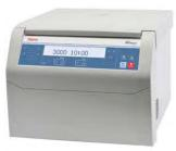
**75007211**: Megafuge 8 ventilated benchtop centrifuge Max Capacity 4 x 145 mL (with TX-150 rotor) Max Speed 4,500 rpm (with TX-150 rotor) Sound Level <58 dBA (with TX-150 rotor) 230 V, 50/60 Hz
