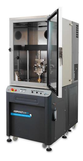
**79-PV72Q02/I2**: AsphaltQube, 15 kN modular electro-mechanically operated asphalt mix tester with inbuilt IMACS2 controller 208-230V/50-60Hz/1ph
