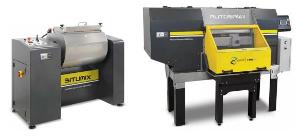
**77-PV0077/CR**: BITUMIX - Automatic laboratory mixer 30 litres capacity Complete with mixing tool with removable and adjustable blades 380V/50Hz/3ph
