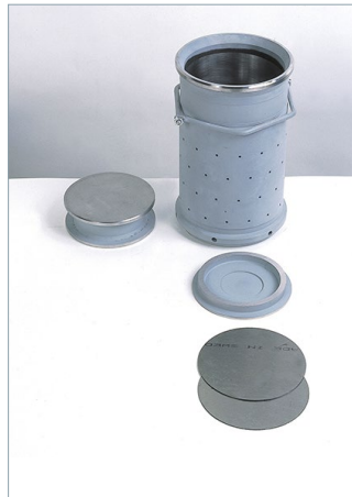
78-PV0250/10, 150mm dia. mould with holes for bituminous emulsion cold mix compaction
