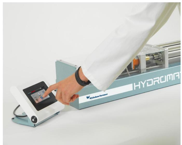
*The control panel is removable and can be located according to user's preferences and needs*
